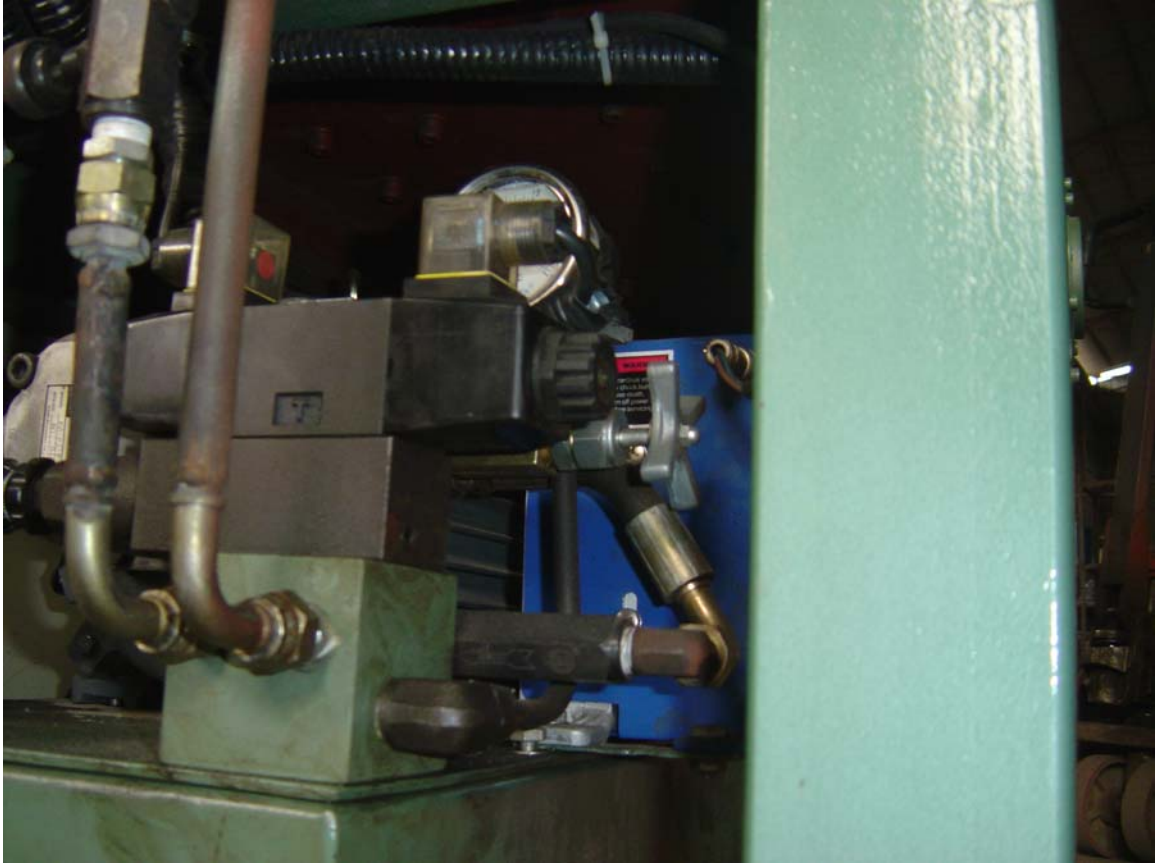
This is another view of the Directional Control Valve and the Main Pressure Valve Assembly of the Power Unit.
